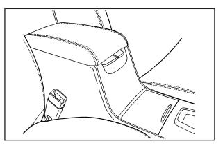
If your vehicle has a full floor console it has two storage areas. To access the upper tray storage, lift the left lever located in the front of the armrest lid. To access the lower storage area, lift the right lever. If your vehicle has a center seat console it will have two storage areas. To access the upper storage area, press the button located on the front of the armrest and lift the armrest lid. To access the lower storage area, pull the strap located behind the cup holder.
